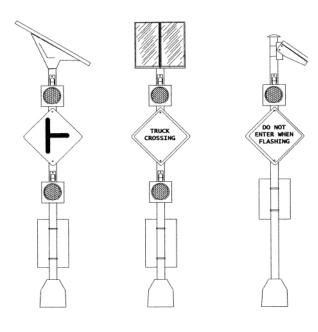
self-contained flashing beacon power system. Both the solar array and the battery bank will be designed to meet your project requirements based on solar radiation for your site.
