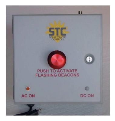
The 80FSXTAC-1 is a radio-activated, wall unit designed to be mounted in the fire station's truck bay. It includes a red mushroom button assembly to allow easy activation of the flashers located on the roadway in front of the fire station. It has status lamps for power, a 27Mhz license-free radio transmitter with a 5W RF output, and audio feed back when the button is depressed.
